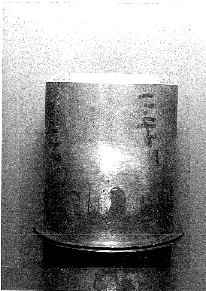
Figure 3.5 Notch produced by weld flash.
