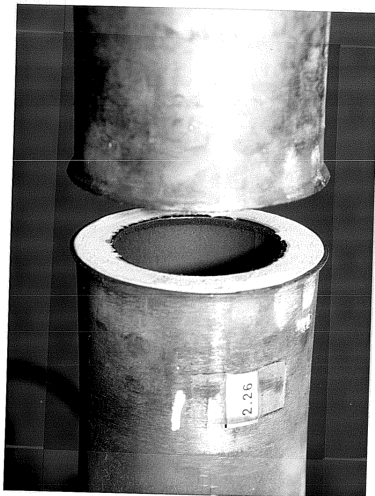
Figure 4.2 Fracture surface of weld fabricated before hydraulic modification.
